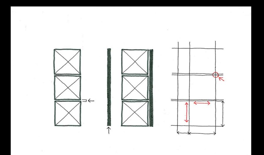
a series of crosswalls divide the units, and a separating tartan grid allows services to be positioned logically with ease of access
