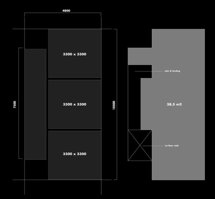
the plan allows for a staircase/kitchen core to be placed centrally and (if necessary) fire protected allowing ease of escape
