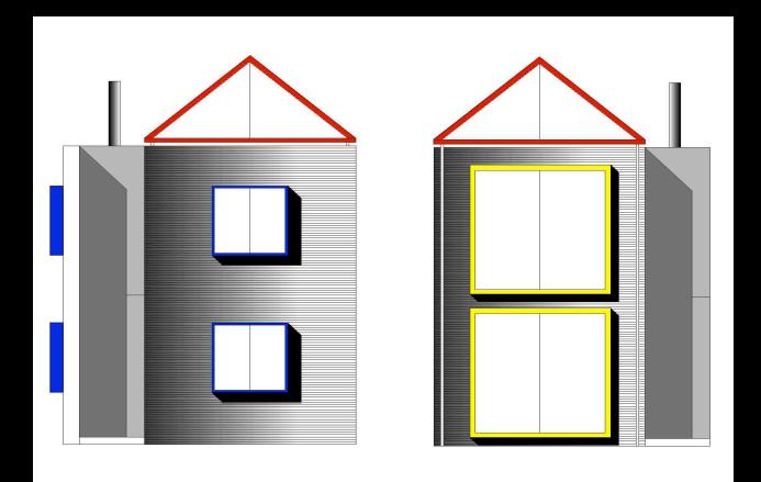
area calculations TYPE 1 (2 storey) are based on internal floorspace minus 1 staircase, 1 landing & 1 double height void
